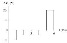
Assess: The potential difference is proportional to the negative slope of the current versus time graph.
